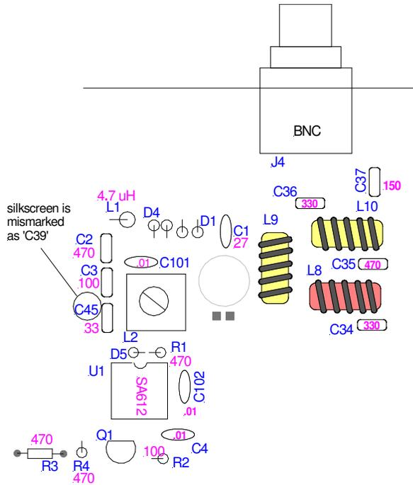
Install 1N4148 diodes at D1, D2, D3 and D4. Match the installation polarity as shown on the silkscreen and pictorial drawing.
