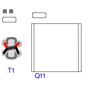
the board. . Make sure that the heat sink is aligned parallel with the board before tightening the nut. ***Tighten cautiously- the nylon screw threads will strip at the torque typically used for steel hardware.*** Solder Q11's leads into place.
