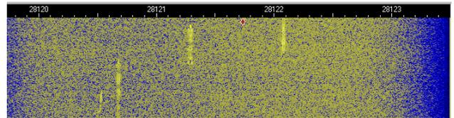
*/ This image was taken with the 'microphone' gain at maximum, an antenna connected, and C38 adjusted to center the 'yellow band' onscreen. (The wide yellow band is considerably brighter with a strong noise source.)*
