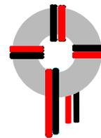
*Note the way the color-pairs are arranged as they proceed around the core.*
