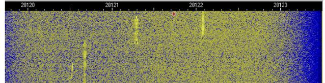
*/ This image was taken with the 'microphone' gain at maximum, an antenna connected, and C38 adjusted to center the 'yellow band' onscreen. (The yellow band is considerably more apparent with a strong noise source.)*
