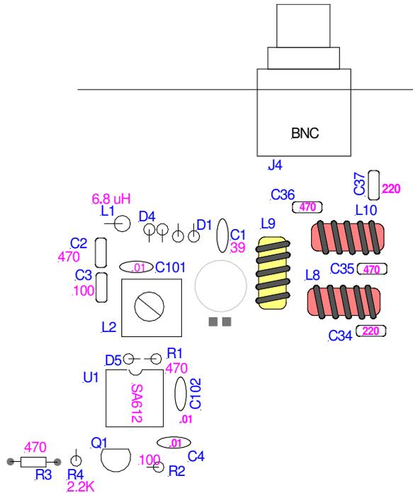
□ Install 1N4148 diodes at D1, D2, D3 and D4. Match the installation polarity as shown on the silkscreen and pictorial drawing.
